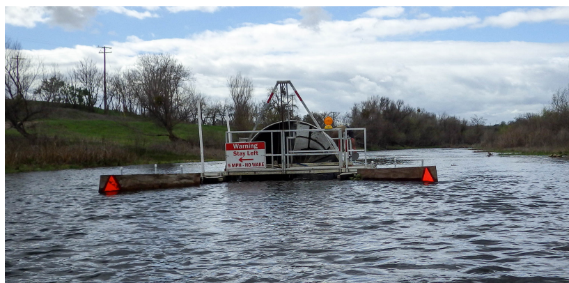
Figure 2. Waterford RST with “wing” structures on upstream end of pontoons.
